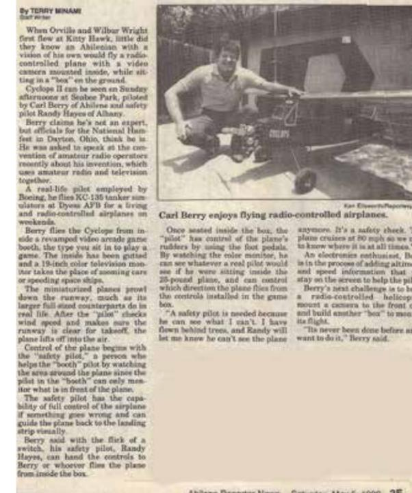
System. This was first test flown back in 1989, and video at a publicly sanctioned flying event in 1993 or 1994 shows Carl demonstrating his cockpit – the enclosure from an old Sega arcade machine. His plane, an 8 ft long twin gas plane weighing 15 kg with a 10 ft wingspan needed to be large to accommodate the bulky CCD security camera.
