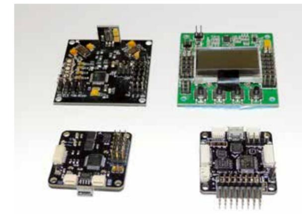
The evolution of flight controllers (From top left). The original (pre-build) KK board, the HobbyKing produced KK2, the extremely hard to find Open Pilot Copter Control board, and finally up to date with an SP Racing F3 board
